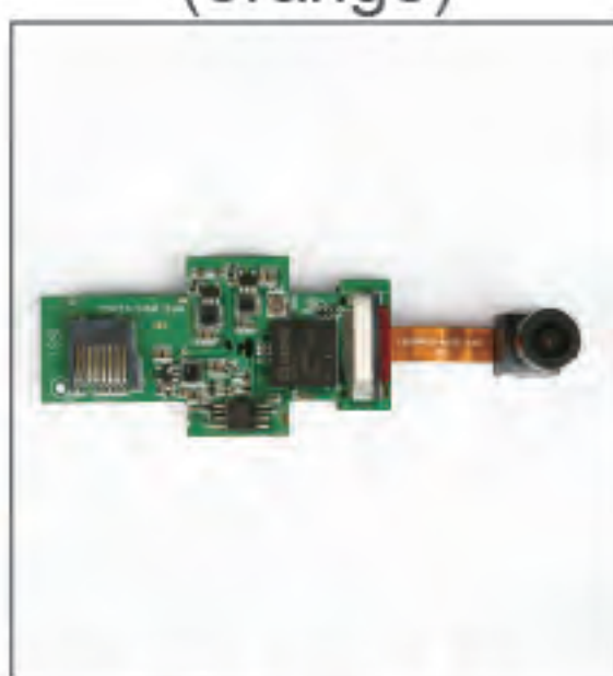
H216A-03 1080P Camera module/VTX
